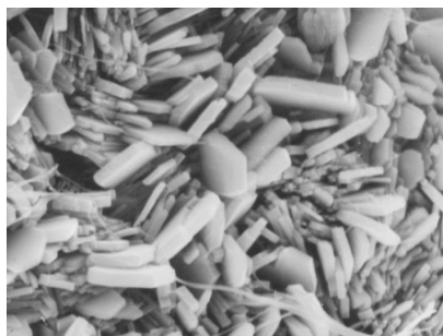
FIG. 2 SEM micrograph of raw clinoptililite-rich tuff from Nižný Hrabovec (East Slovakia); magnification 3700 X
